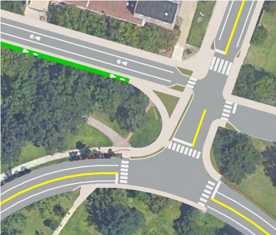
All Stop and Pedestrian Upgrades at Schenley Dr & Tech St
